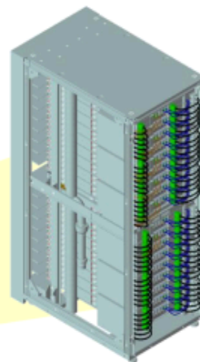
19-inch rack 216 nodes
